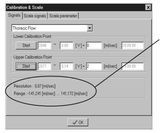
Here the resolution and the maximal range for the signal is displayed. It is important to check these values. If the resolution is not as good as required (less than 0.1 ml/ sec) the gain of the amplifier must be increased, so that higher values for the upper calibration point are received. If the calculated range seems too small, the gain of the amplifier must be reduced. If gain has been changed also redo the lower calibration (see 7.3.2)
