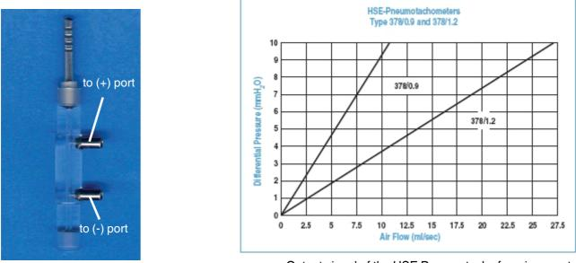
Output signal of the HSE Pneumotachs for mice or rat
