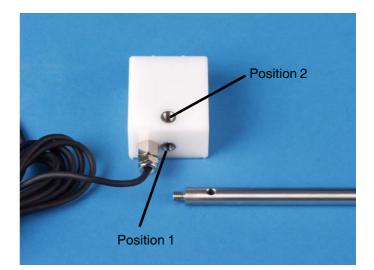
driver can be introduced to tighten the rod on the transducer.
