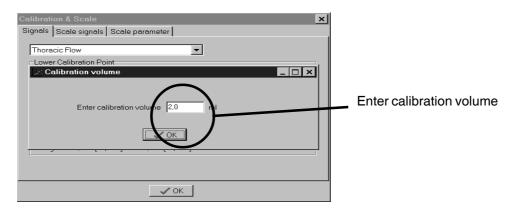
Prepare a syringe, filled with the choosen volume of air (in our case 2 ml for a rat pneumotach (0.5ml for a mouse pneumotachometer) connect the syringe to the pneumotach or to the plethysmographic box.
